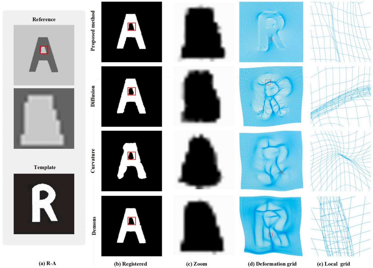
Fig. 8. Registration results of R-A images across four methods. (a) reference and template images; (b) registered images using optimal parameters (Proposed method: \alpha = 0.45, \beta = 0.001, \gamma = 0.01, \lambda = 0.1, \rho = 1.02, n_r = n_t = 40 ; Diffusion method: \alpha = 0.0001, n_r = n_t = 8 ; Curvature method: \alpha = 0.0001, n_r = n_t = 20 ; Demons method: \alpha = 4 ); (c) zoomed regions of interest; (d) deformation grids; (e) local enlargement of deformation grids.
