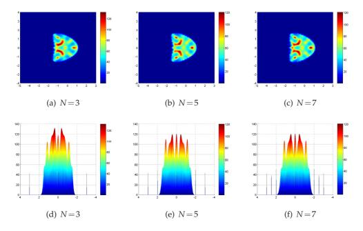
Figure 6: Reconstruction of kite-shaped extended obstacle and N point-like scatterers lying around with  $\alpha_i = 1$ .
