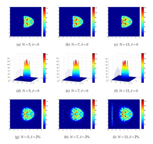
Figure 5: Reconstruction of kite-shaped extended obstacle and N point-like scatterers lying on the line segment  $\{(x_1, x_2) \in \mathbb{R}^2 : x_1 = -4, x_2 \in [-3,3]\}$  with  $\alpha_j = 1$ .
