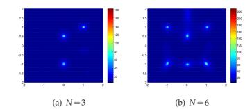
Figure 1: Reconstruction of N point-like scatterers using MUSIC algorithm with  $\alpha_i = 1$  and M = 10.
