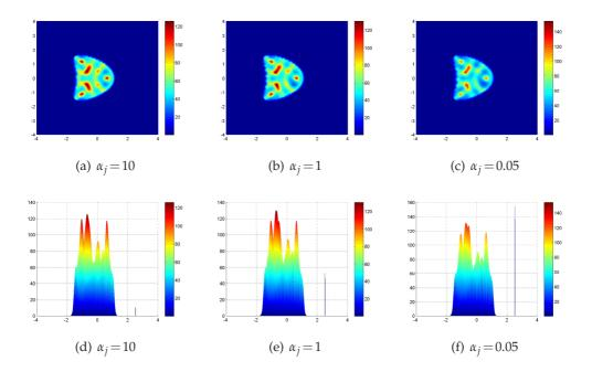
Figure 7: Reconstruction of the kite-shaped extended obstacle and one point-like scatterer with different scattering coefficients.
